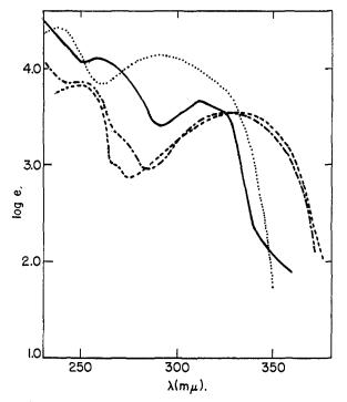
Fig. 1.—Ultraviolet spectra in 95% ethanol of III, freshly prepared (-----) and after 24 hours (-----); of an equimolecular mixture of o-aminobenzamide and phenylboronic acid (------) and of IV (....).
